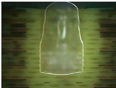
L1-L15 NPTH Depth control (2.0mm)
